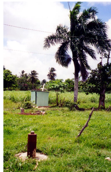
Well #7 in the Los Marenos well field. One of the MP TROLL 8000s is mounted in a nearby well with an identical surface completion.
