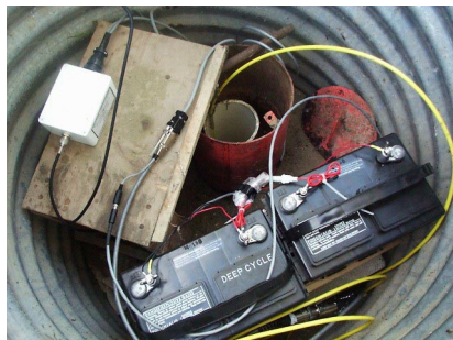
Equipment installed at the wellhead (clockwise from white box on left): proprietary telemetry link, instrument communication cable, PVC well casing with 2" inner casing enclosing TROLL, and batteries to power the telemetry link and the TROLL. All components are completely enclosed and locked.
