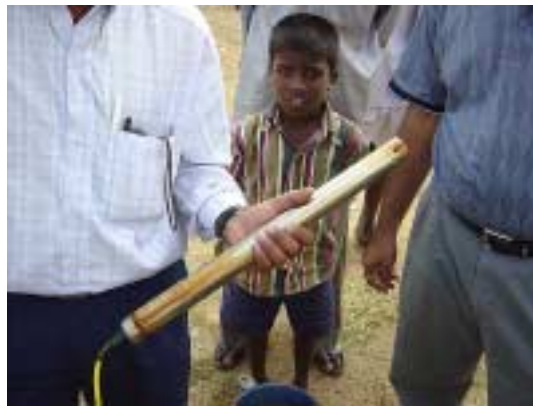
Heavy deposits of rusted well casing material on the TROLL's stainless steel sensor housing can cause damage to the sensor.
