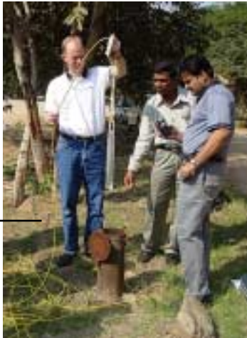
Use of a Water Barrier Kit creates a fresh water barrier around the unit, protecting it from chemical reactions with the rusted materials.
